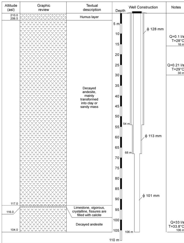
Fig. 2. Lithological profile and construction of well B-1 (after MILOJEVIĆ, 1973, simplified).
