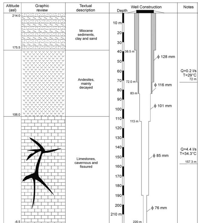
Fig. 3. Lithological profile and construction of well B-2 (after MILOJEVIĆ, 1973, simplified).
